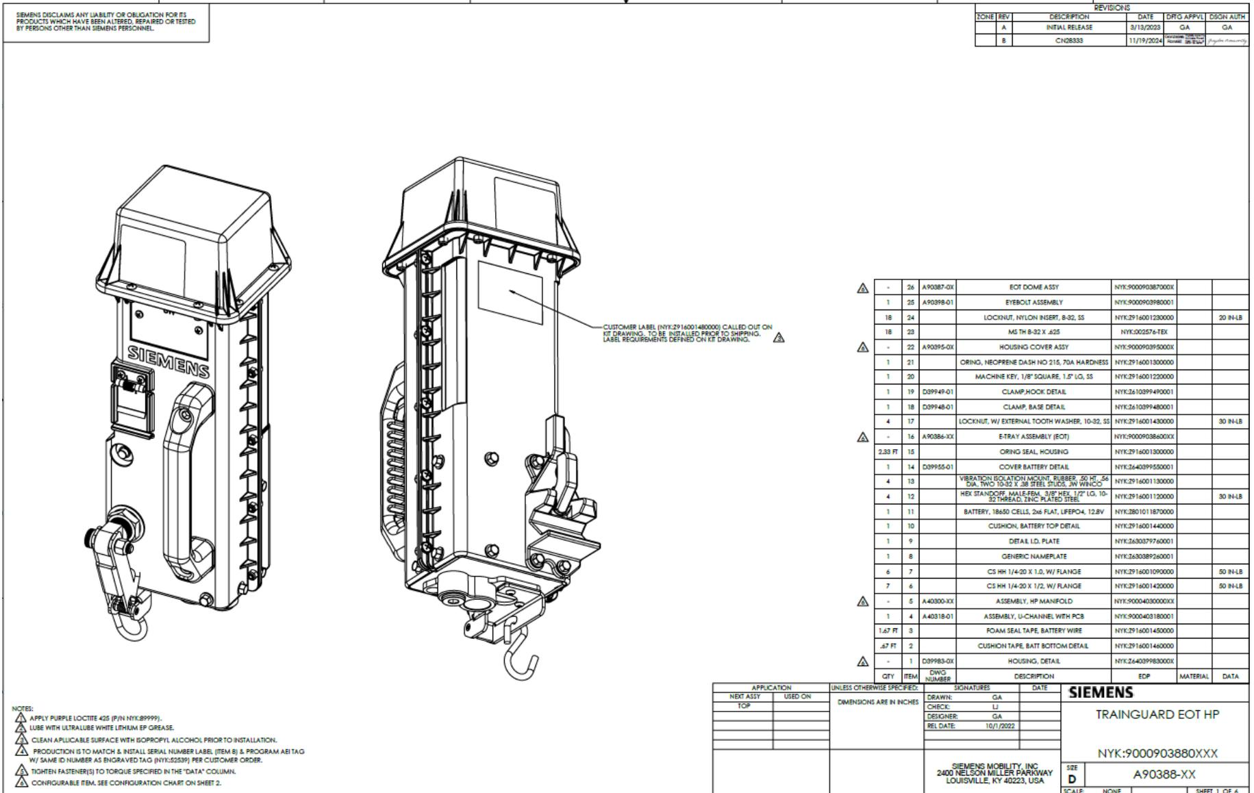
Figure 9-6 Main Assembly with HP Manifold, A90388 Sheet 1
