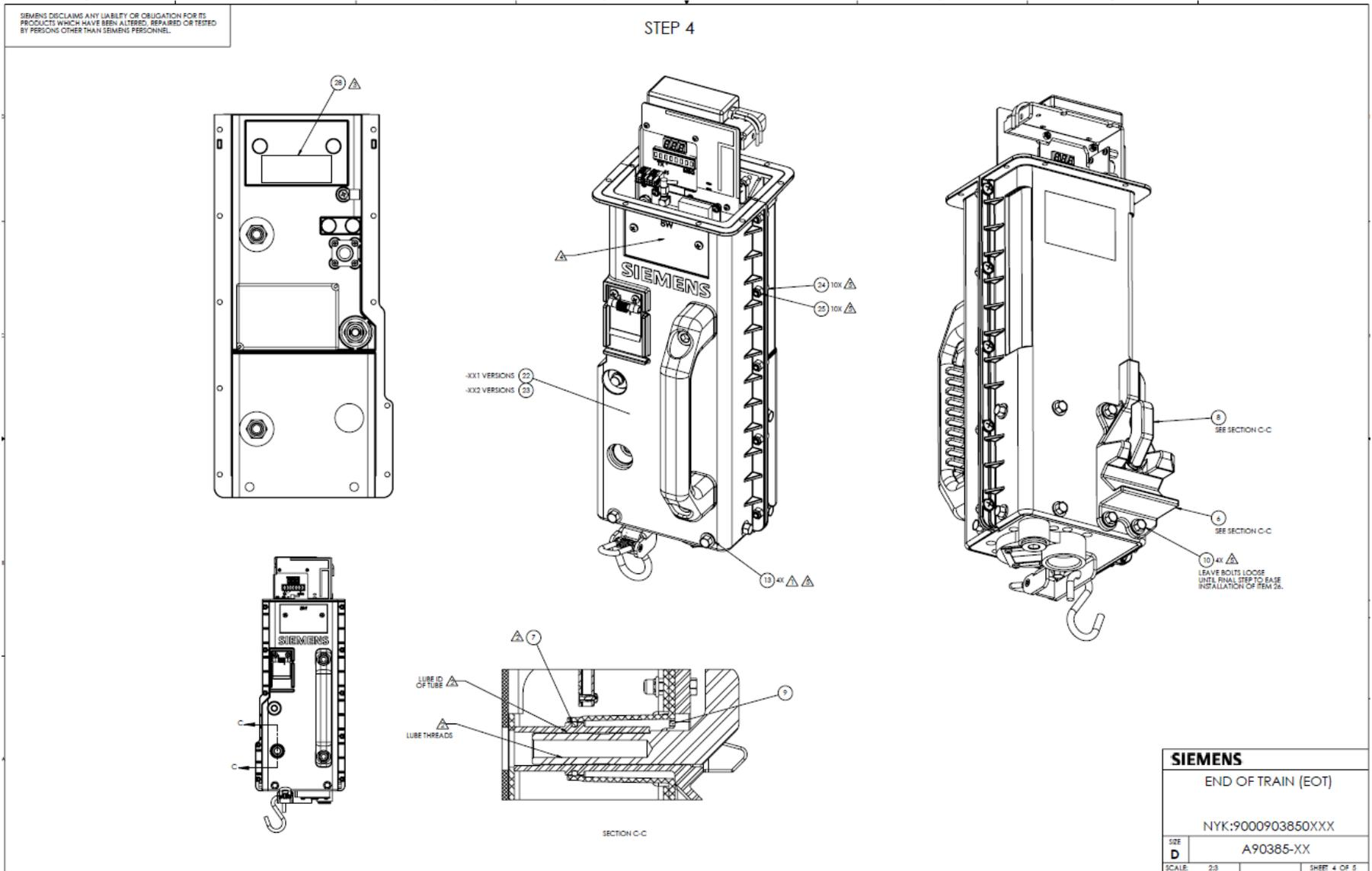
Figure 9-4 Main Assembly, A90385 Sheet 4
