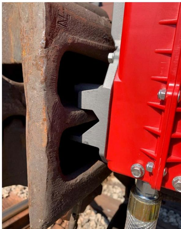
**Figure 2-3 Clamp Groove on Coring Hole Web**
