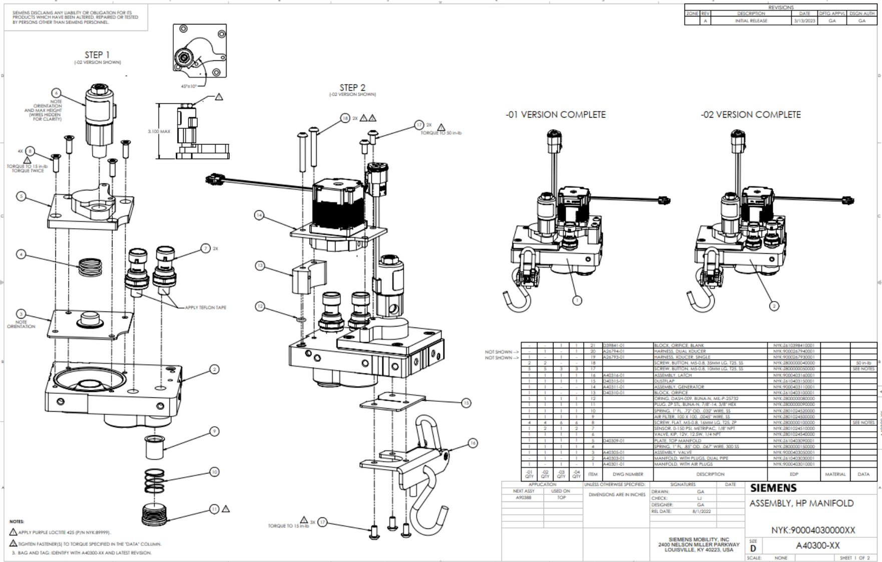
Figure 9-15 High-Powered Manifold Assembly, A40300
