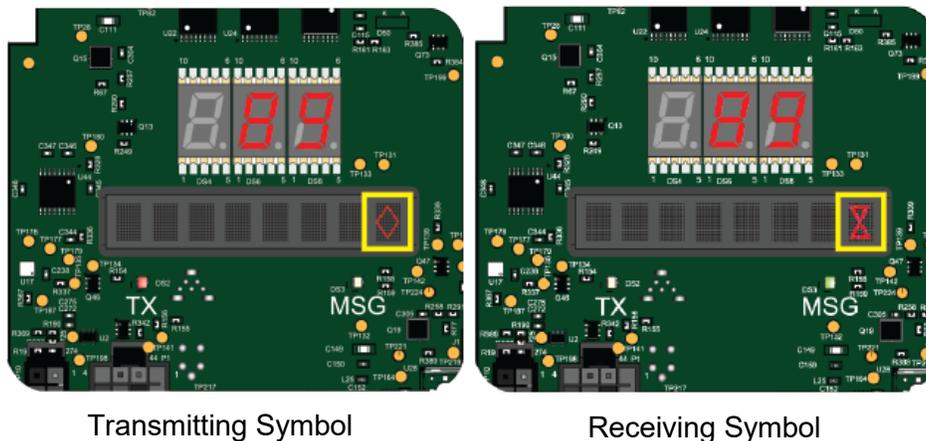
**Figure 3-8 Messages TX / RX indicators - Transmitting (Left) Receiving (Right)**
