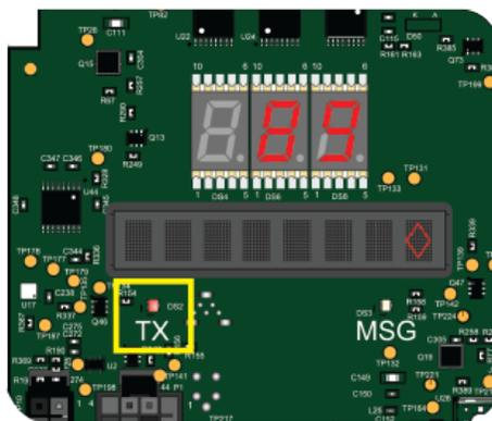
Figure 3-6 Transmitting LED
