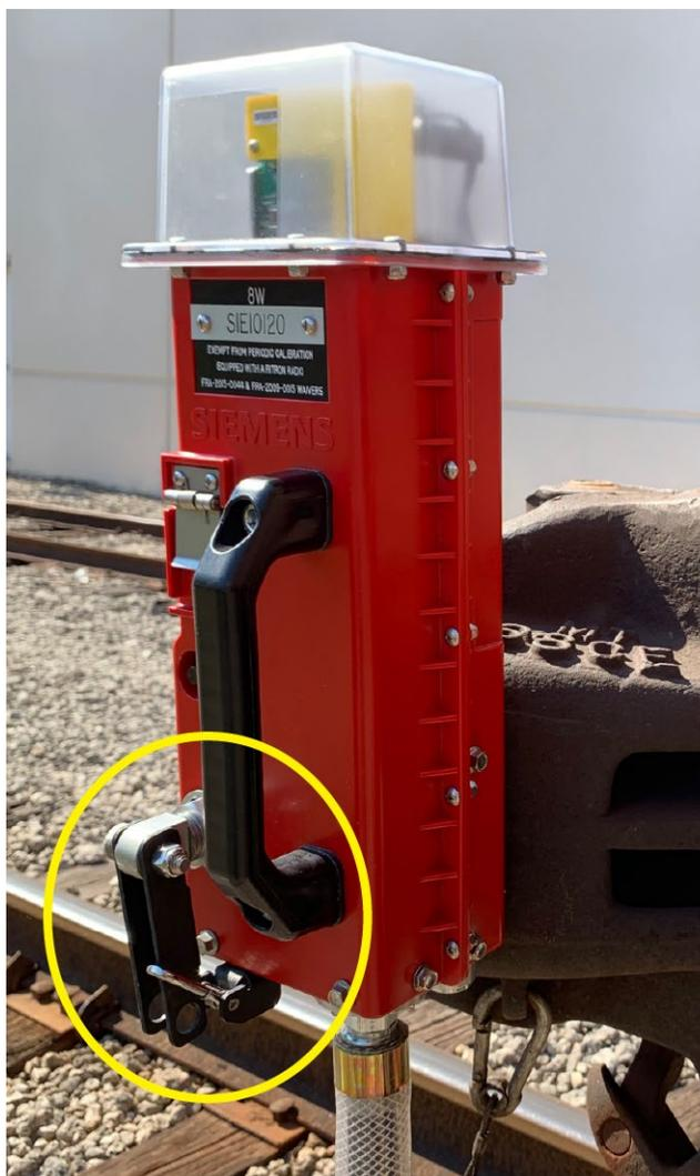
Figure 2-1 Unlatching the Crank Handle
