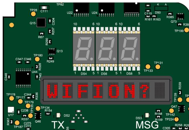
Figure 4-3 Pushbutton Wi-Fi On Message
