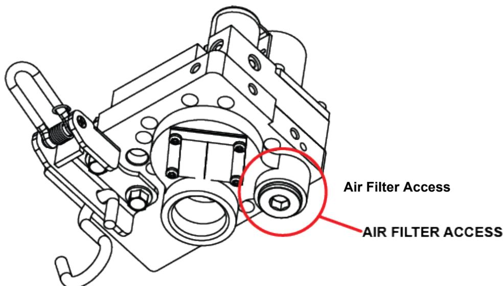
Figure 3-9 Air Filter Access Location (Standard Manifold)
