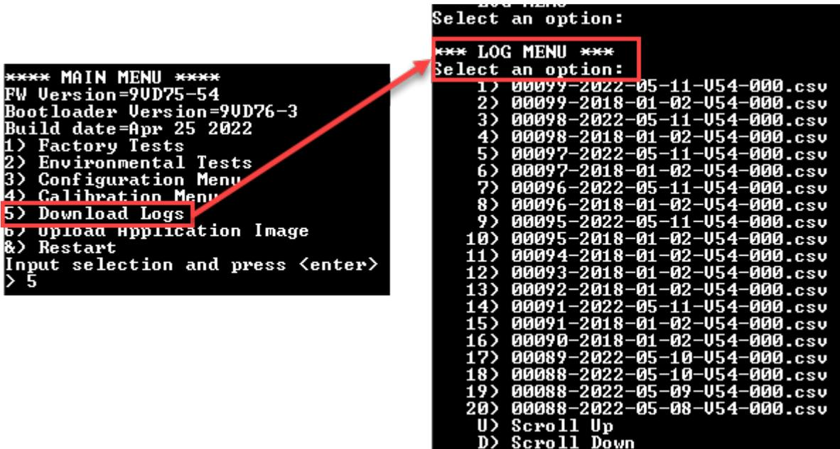
Figure 6-4 Access Logs Via Serial Terminal Interface
