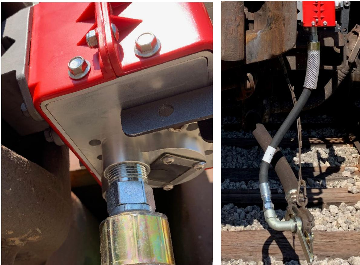
**Figure 2-5 Coupling the EOT Air Hose**
