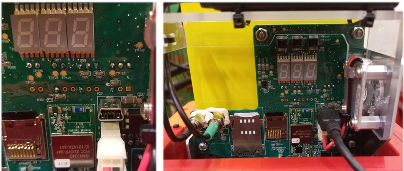
Figure 4-16 Mini USB Connection Point
