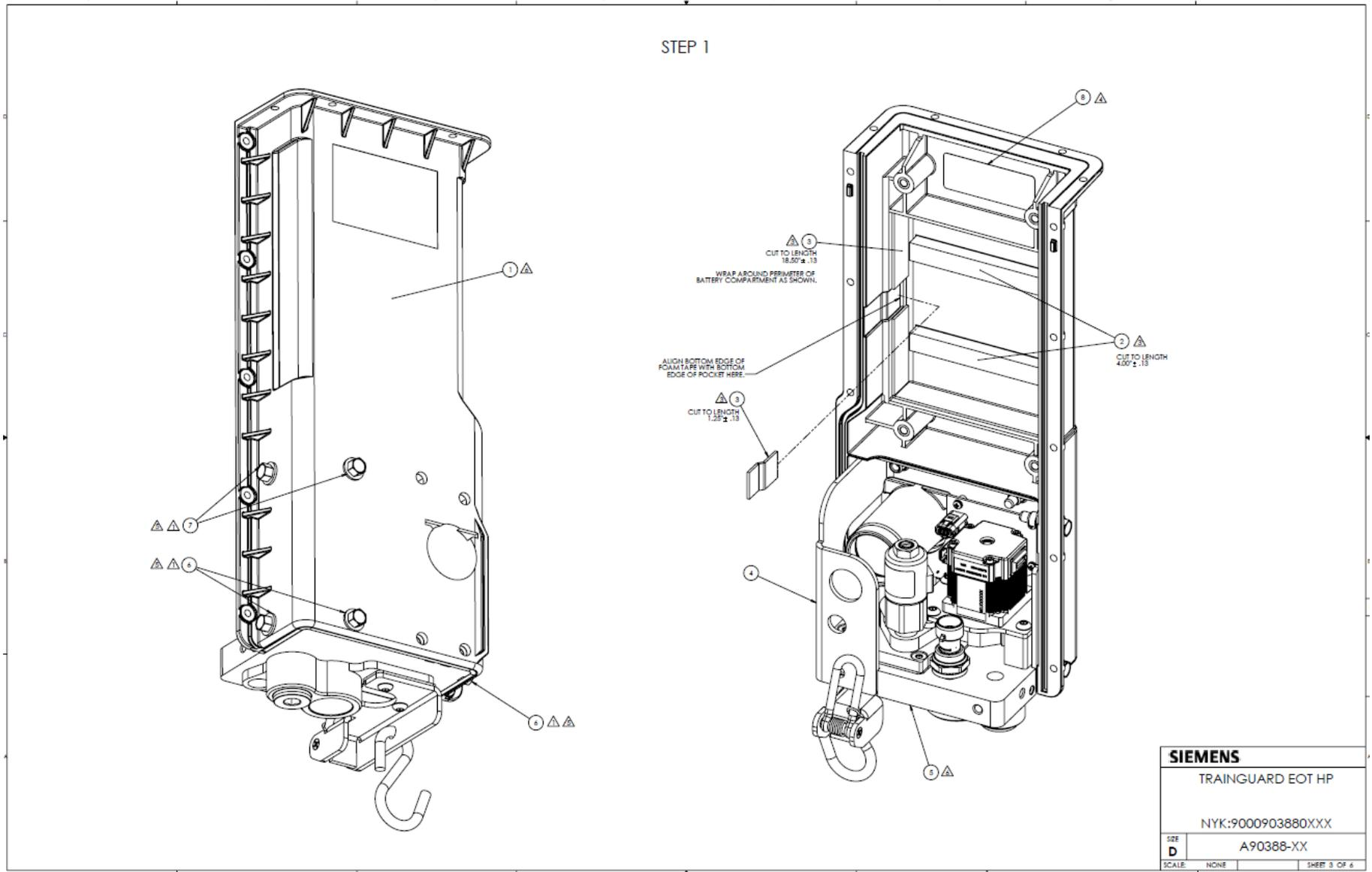
Figure 9-8 Main Assembly with HP Manifold, A90388 Sheet 3
