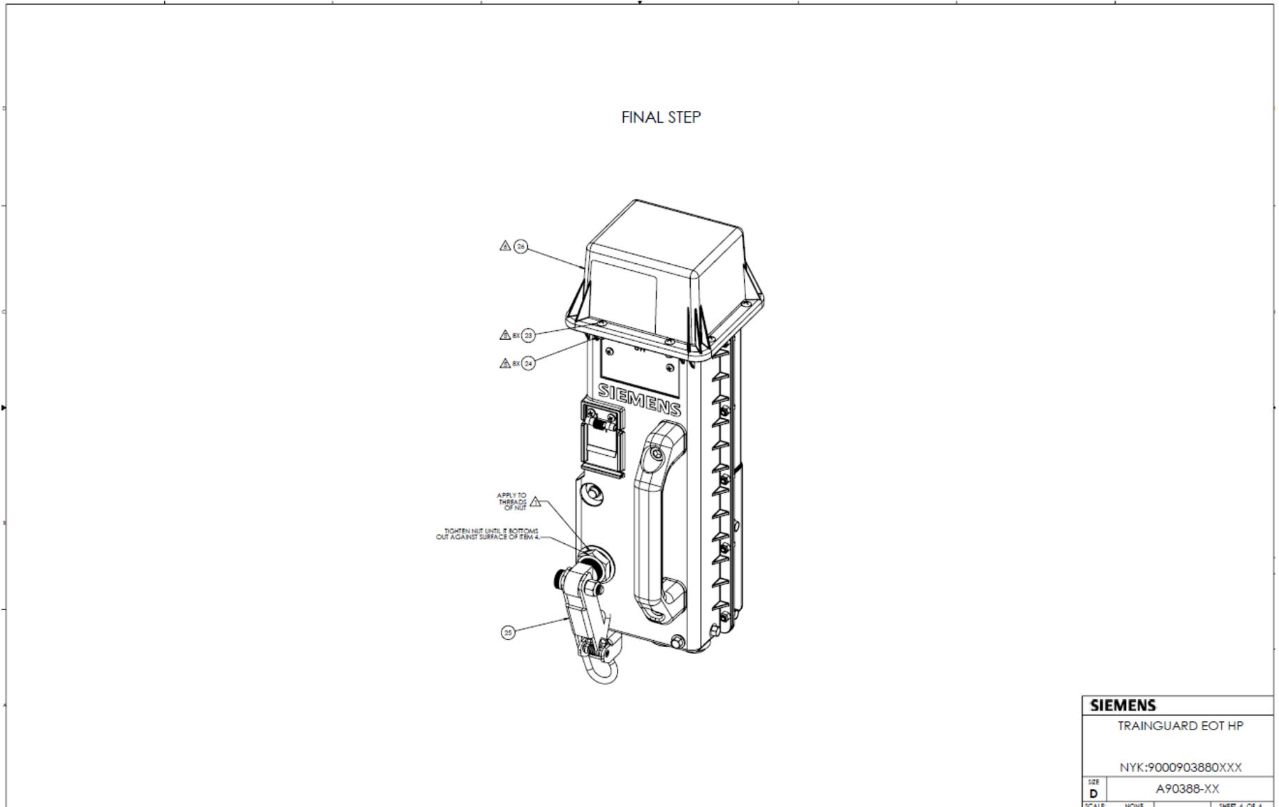
Figure 9-11 Main Assembly with HP Manifold, A90388 Sheet 6
