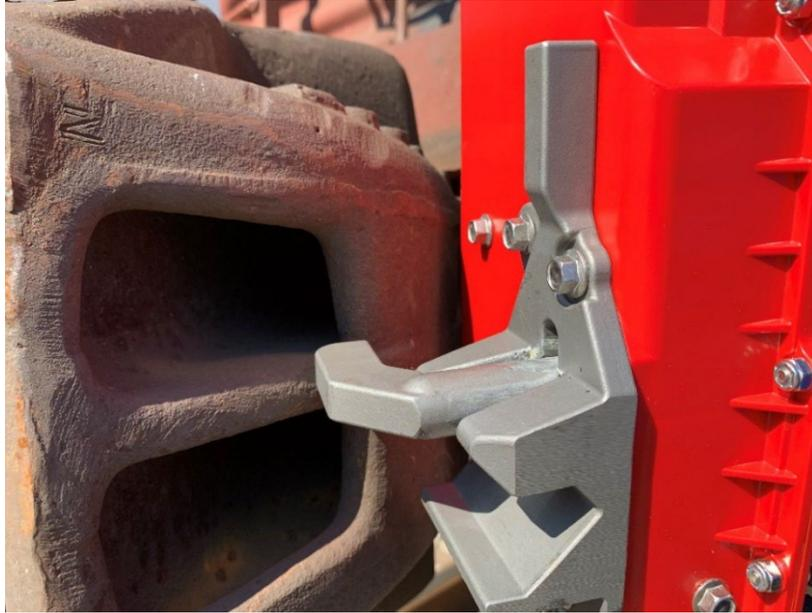
**Figure 2-2 Locking Arm in Horizontal Position**
