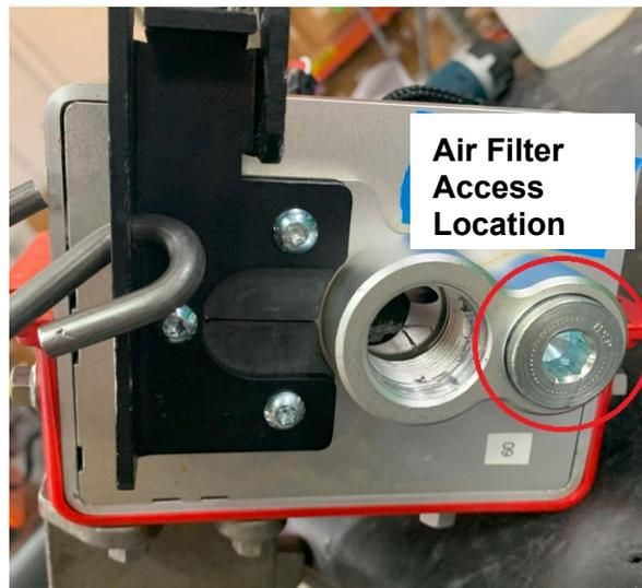
Figure 3-10 Air Filter Access Location (HP Manifold)
