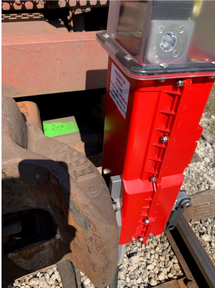
**Figure 2-4 Installed EOT**
