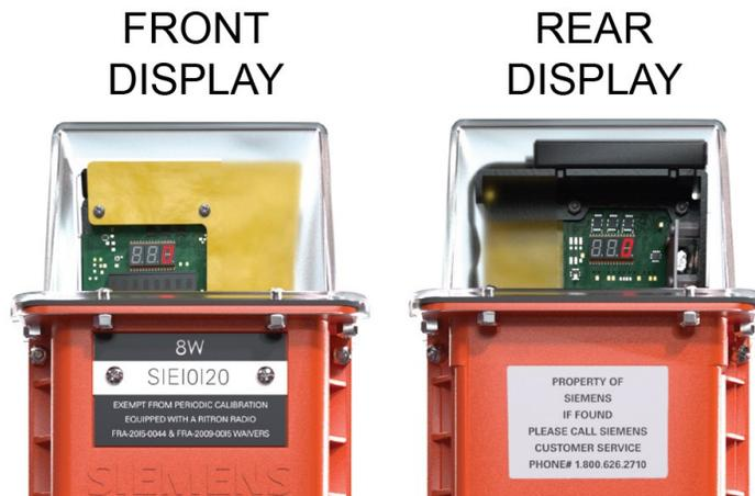
Figure 1-4 Front and Rear Display
