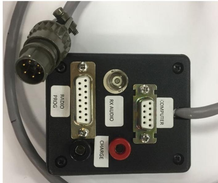
Figure 4-18 Charge Port Adapter
