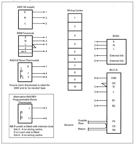
All wiring to be rated @ 240v and earthed as required.
