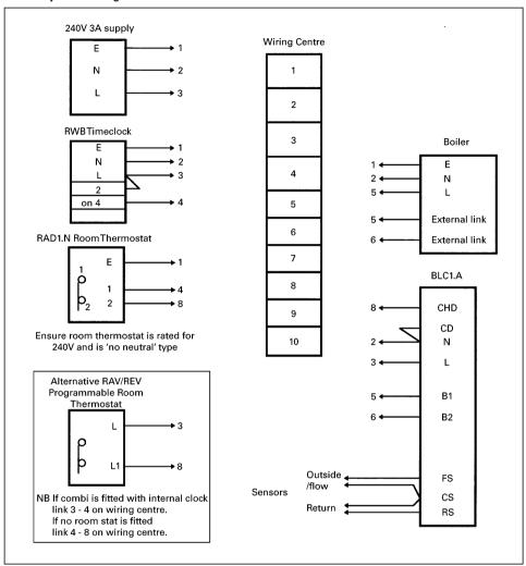
All wiring to be rated @ 240v and earthed as required.
