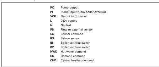
All wiring including wires to sensors should be 240V rated and all components earthed as required. Wiring (except sensors) should be run to a wiring center and the minimum number of links added to the BLC1.A.
