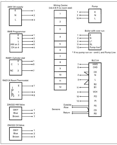
All wiring to be rated @ 240v and earthed as required.
