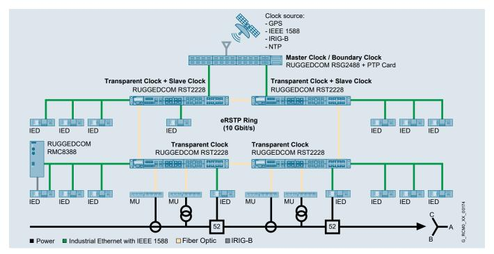
Up to 24 modern IEDs or other IEEE 1588 slaves can be connected directly to the RUGGEDCOM RST2228 via Fast Ethernet or via Gigabit/s ports.
