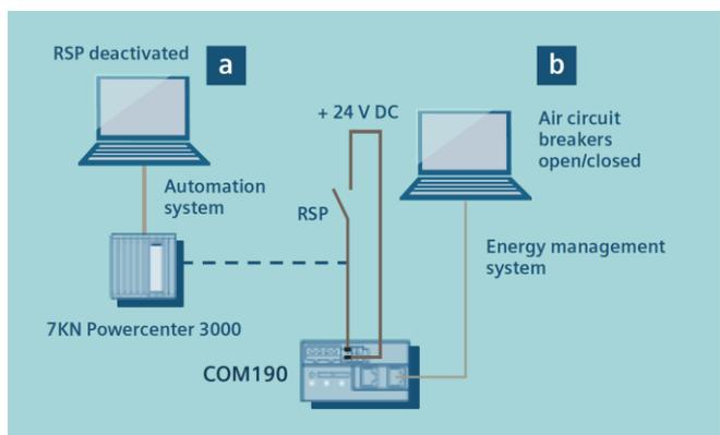
Temporary activation and deactivation of remote switching protection (RSP) for the 3WA air circuit breaker.
