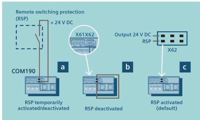
Activation of remote switching protection (RSP) for the 3WA air circuit breaker.
