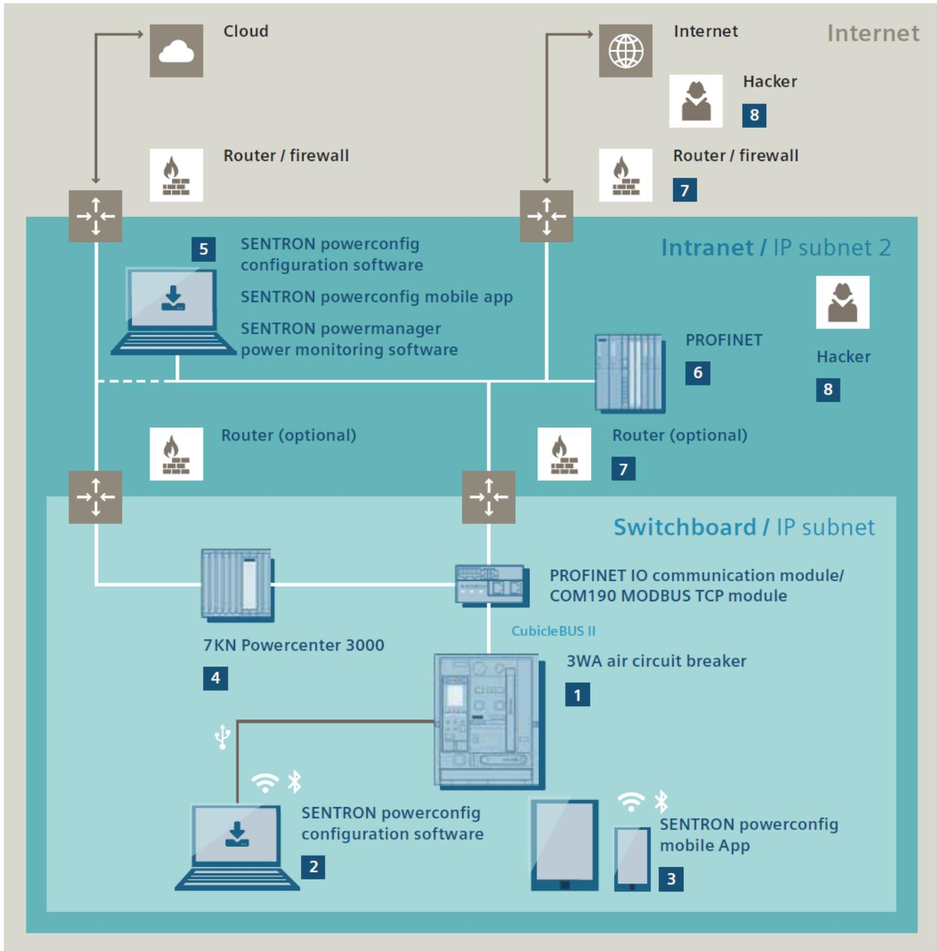
A cybersecurity concept using the 3WA air circuit breaker as an example.
