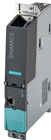
CONTROL UNIT CU320-2 WITH PROFIBUS or PROFINET interface. The interface also contains digital and analog inputs and outputs. Extension cards can be installed enabling communication via CANopen or EtherNET / IP.
