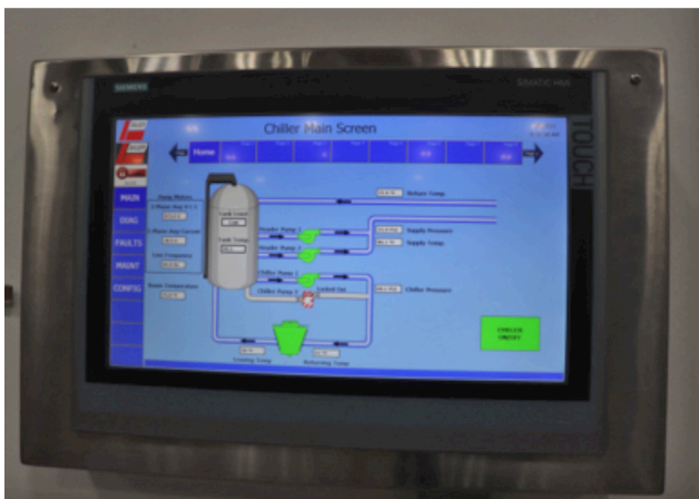
The 19-inch SIMATIC HMI Comfort panel is mounted outside the Bauer engineering office door, so staff can easily check the status of various testing stations.
