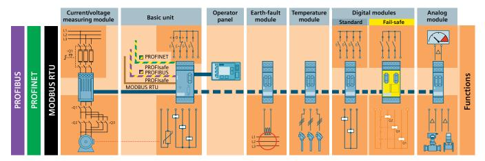
With SIMOCODE pro you get the full range of features. The motor management system can be connected to all important communication systems – PROFIBUS and PROFINET as well as OPC/UA and Modbus RTU.
