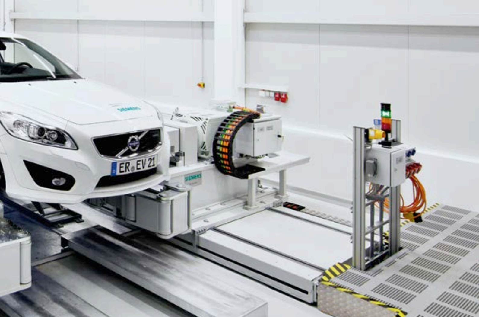
Application example for an automated vehicle test bed with CATS flexible
