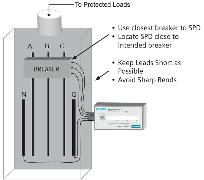
Figure 4: Typical Flush Mount Installation
