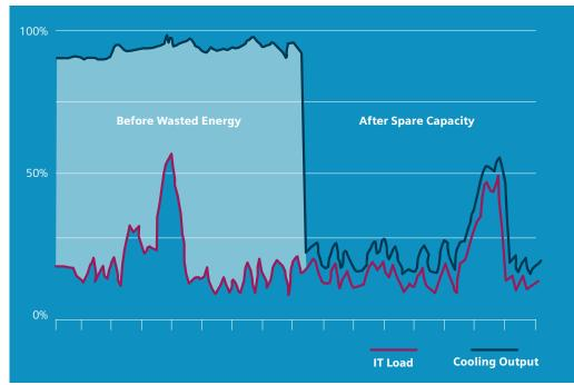
The AI engine uses real-time data to produce algorithms that predict the best level of cooling that will deliver the desired temperature at each sensor.
