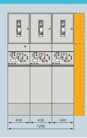
The figure illustrates the space gained for three circuit-breaker panels with low-power current and voltage sensors as against a switchgear with conventional current and voltage transformer technology by the example of the CKW switchgear mentioned as a reference above.
