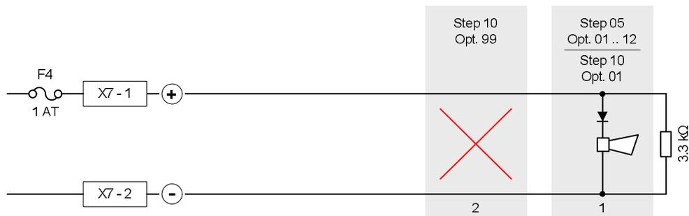
Fig. 22 XC100x-A, monitored control output 1 connection
