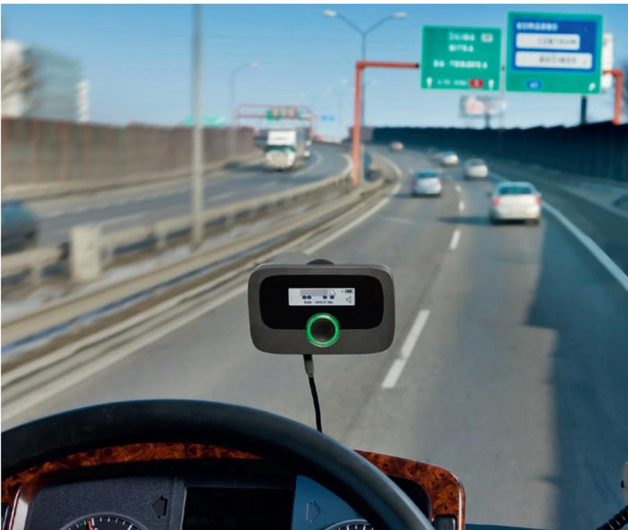
➤ The satellite-based OBU, the core of the solution, is used to detect tollable roads and road segments
