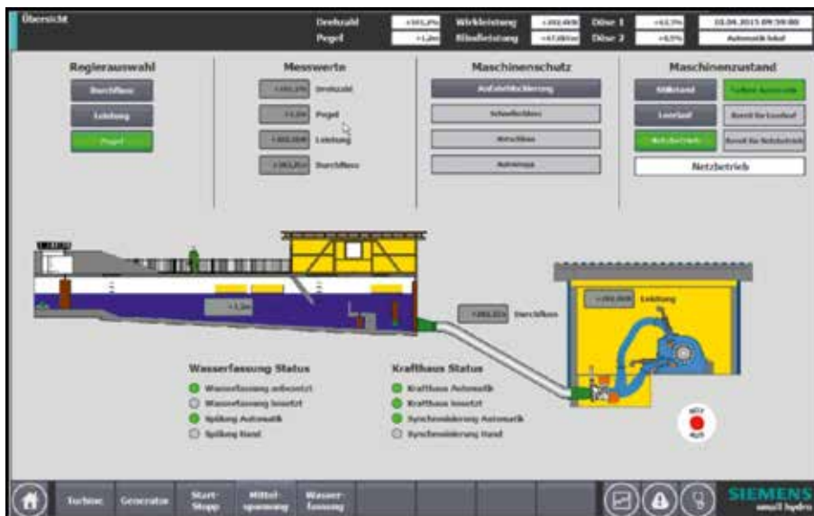
Plant overview of a single unit small hydro power plant (screenshot). The relevant measured data is shown for the plant operation. The operation modes, the selection of the active controller and the unit protection state are clearly arranged and represented.
