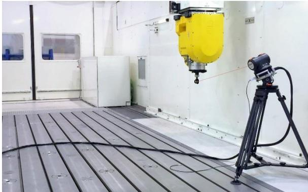
The unique basic principle of measurement with the LaserTRACER: As in the case of the Global Positioning System (GPS), spatial information is obtained by pure distance measurements in space. In the working volume of machine tool, spatial accuracies in the sub-micrometer range can be achieved with largely automated measuring routines.
