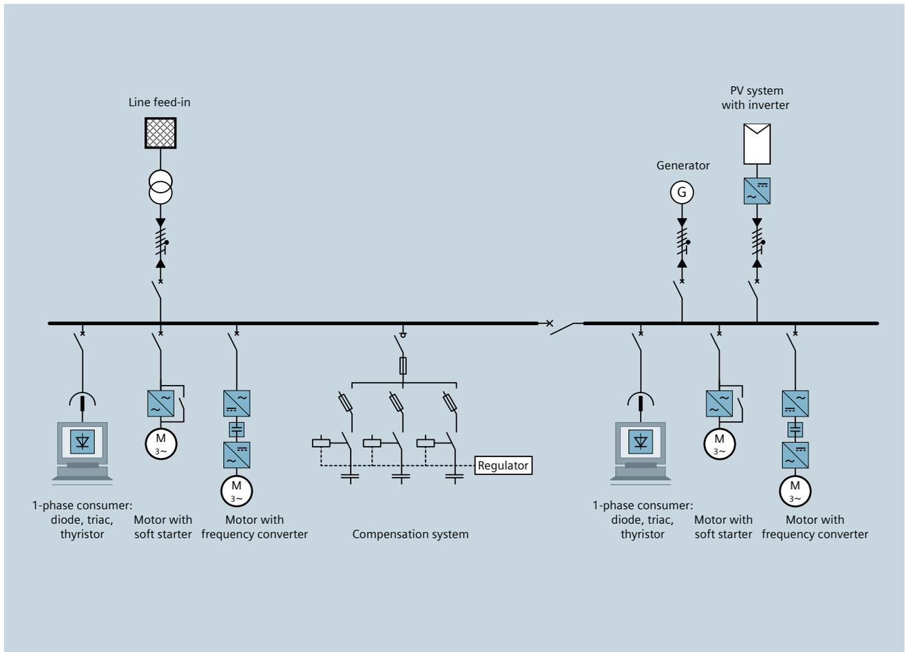
Fig. 3: Distribution grid with non-linear loads, supplied from a distribution transformer and photovoltaic system or a standby generating set and photovoltaic system in isolated operation
