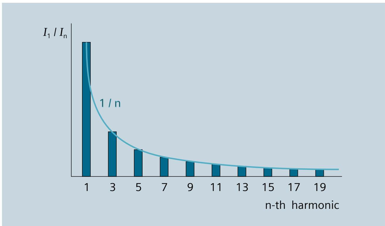
Fig. 5: Harmonics spectrum for a B2 bridge circuit
