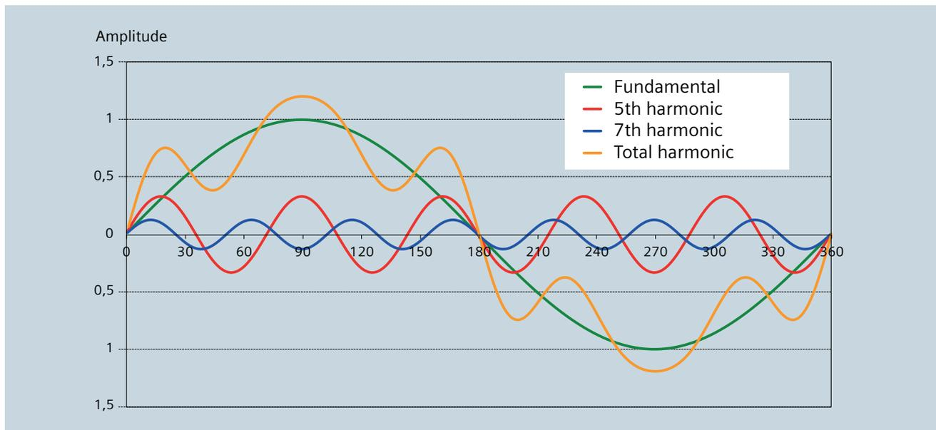
Fig. 1: Impact of harmonics on a sinusoidal fundamental
