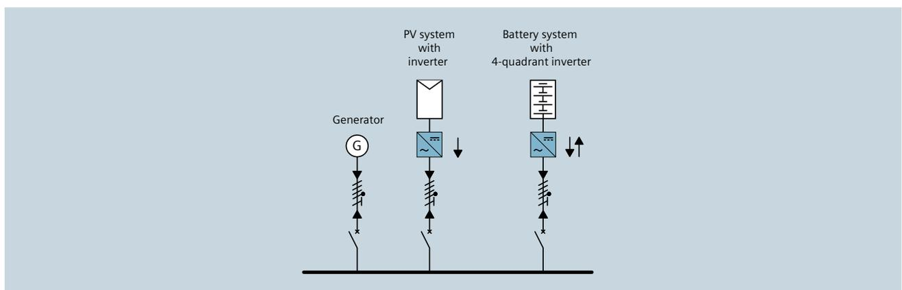
Fig. 9: Power supply in the isolated network with generator, PV system, and battery storage system
