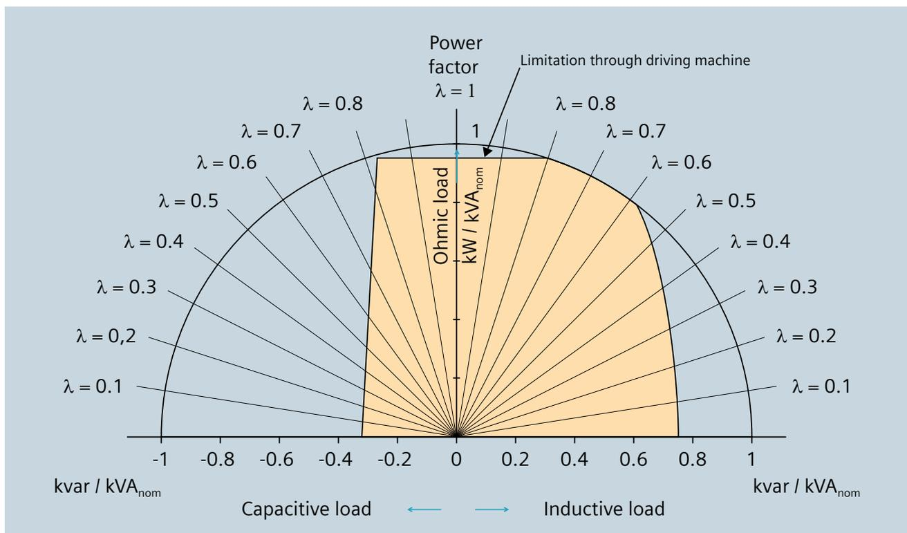
Fig. 4: Example of a generator load curve as Heyland diagram
