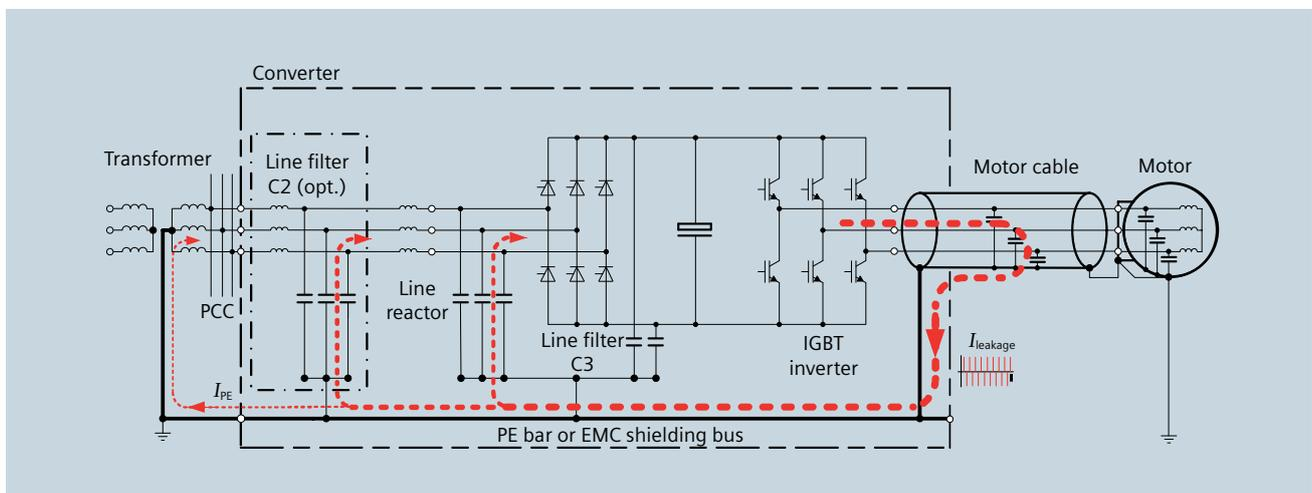
Fig. 7: Filtering of leakage currents in the frequency converter
