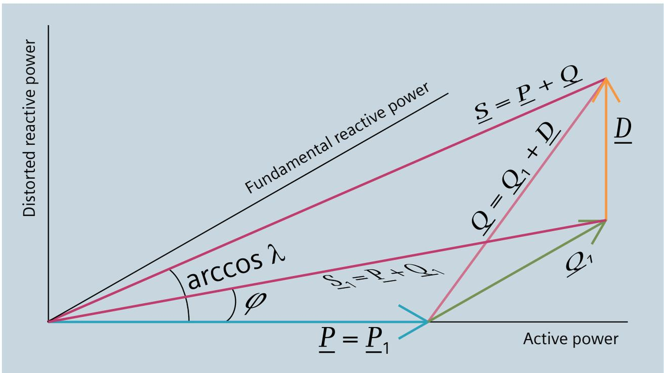
Fig. 2: Vector representation of active power  $P_1$ , reactive power  $Q_1$  for the fundamental, and  $D$  for the distorted reactive power as well as the apparent power  $S$  and  $S_1$  for the fundamental
