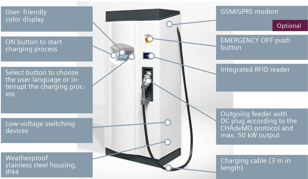
**Fig. 10: Example of a DC fast charging station**
