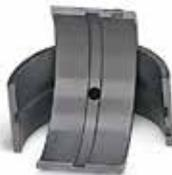
Bearings are horizontally split precision-type tri-metal bronze with micro-babbitt overlay to ensure better heat dissipation, reliability, and increased life; main bearings are identical to crankpin bearings.
