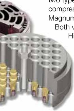
The HOSS compressor uses either solid or two-piece cast iron, steel or aluminum pistons depending upon service conditions, balance and inertia forces. Integral steel pistons and rods may be used in high-pressure applications.
