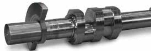
The heavy-duty forged alloy crankshaft is rifle drilled for connecting rod lubrication. The crankshaft is equipped with integral counterweights on the two- and four-cylinder ends to reduce horizontal moments.
