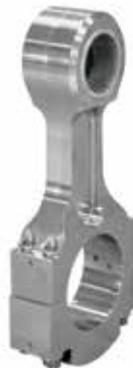
Forged steel connecting rods are rifle-drilled for pressure lubrication and feature high-strength forged ferrule head capscrews with rolled threads. Connecting rod pin bushings are solid bronze with a micro-babbitt overlay.
