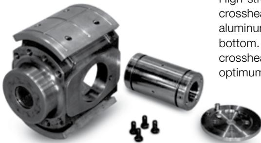
High-strength, nodular iron crossheads feature shim-adjustable aluminum shoes at the top and bottom. Surface-hardened crosshead pins are full floating for optimum reliability.
