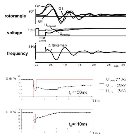
Figure 3: Generator stability and voltage recovery after short circuit
