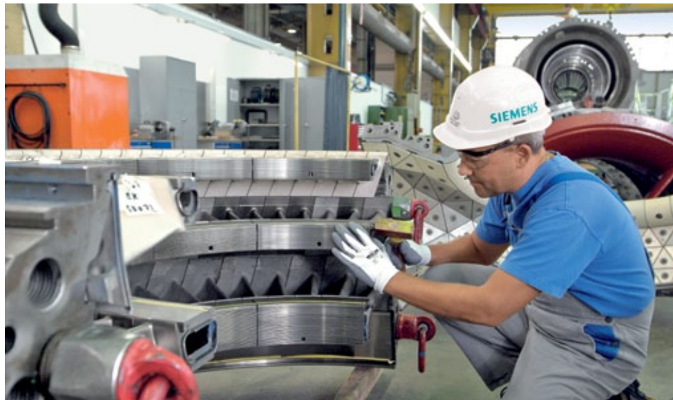
Implementing the modified turbine vanes
