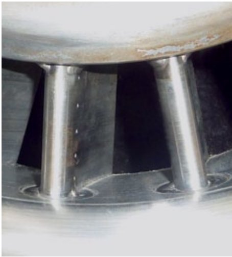
Detail of a model of HR3 diagonal swirler
