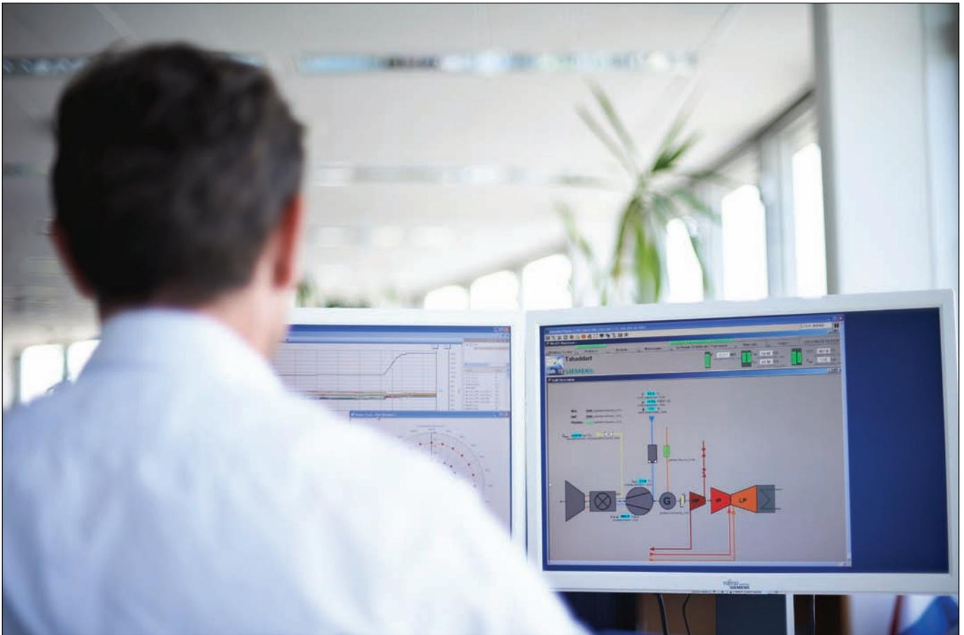
**Remote diagnostics.** Siemens can look at both gas turbine and combined cycle plant operating metrics to see which parameters can be adjusted, with low risk, to restore power or efficiency, or both
