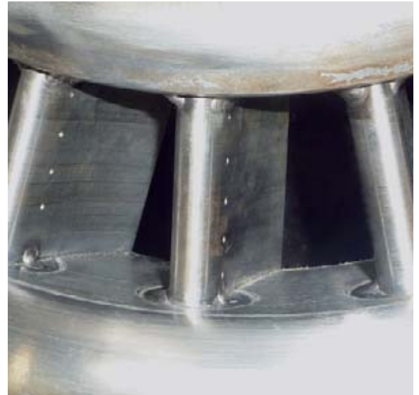
Detail of a model of HR3 diagonal swirler
