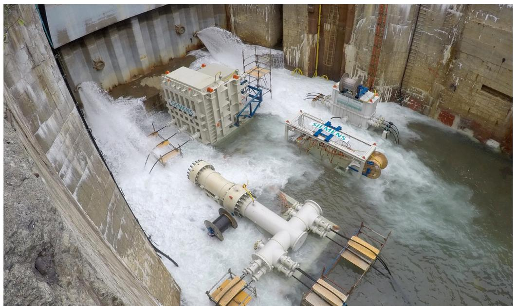
**Figure 1.** Siemens successfully concluded the first phase of its Subsea Power Grid shallow water test in Trondheim, Norway.
