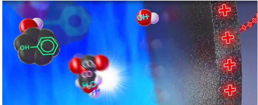
Hydroxyl radicals, formed on the anode, react and oxidize organic compounds in the wastewater stream.
