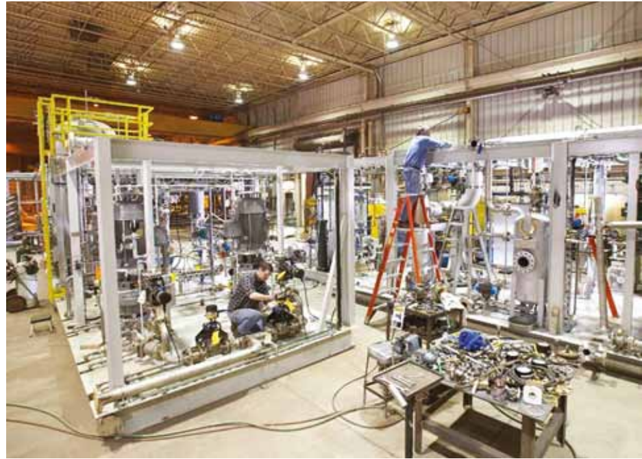
Zimpro® wet air oxidation skids in our manufacturing area.
