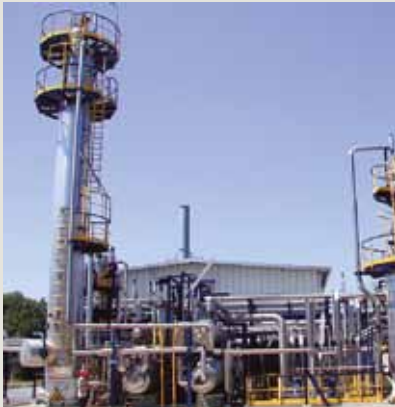
A Zimpro® wet air oxidation system treats industrial waste at Atofina Italia's methyl methacrylate production facility in Rho, Italy.
